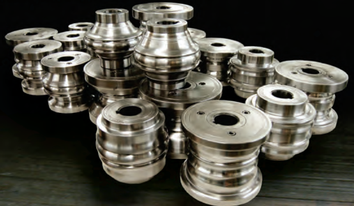
These are the roller dies used by Dennis Carpenter to make 1966-77 Bronco side moldings.
