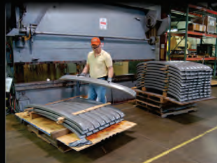
A 150 ton press is used to pierce the mounting holes in our stainless steel 1948-52 Ford truck front bumpers.
