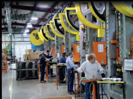
This row of six 185 ton presses is used to stamp stainless steel sheets into Ford car hub caps.
