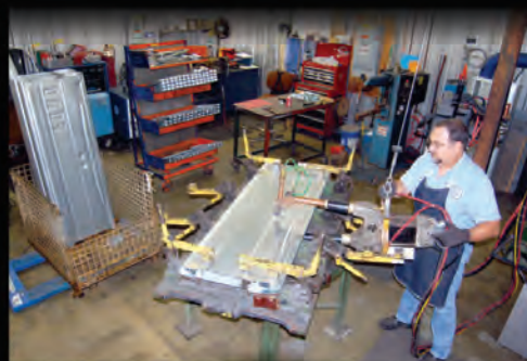
Welding original Ford tooling 1966-77 Bronco tailgates.
