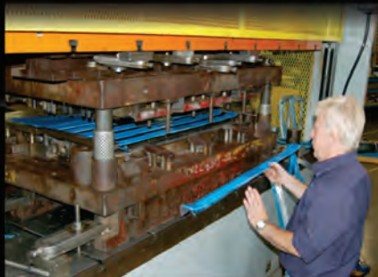
Some scuff plates are made using progressive dies that perform 7 operations per 1 stamping cycle.
