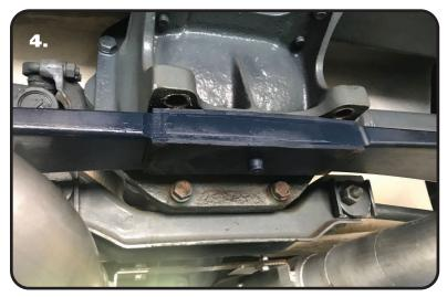
**4. 63-78 CORVETTE WITH 2 1/4" LEAF SPRING!** Position the leaf spring in the OEM location with the ends of the leaf spring pointing downward. THE CENTER LOCATING PIN NEEDS TO BE INDEXED INTO THE HOLE OF THE HOUSING.
