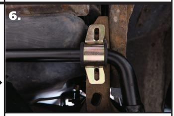
**6.** Slide the Sway Bar into position on the car. The sway bar is installed in the OEM location. You may need to move the bushing/straps on the sway bar to line them up with the OEM mounting holes.
