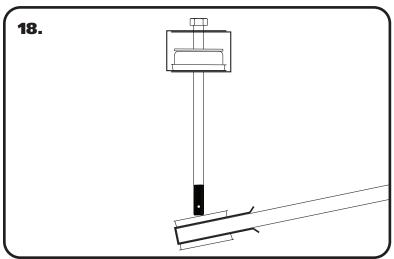
**18.** Insert the 1/2"-20 x 9 1/2" bolt in the leaf spring bushing. The bolt will go in through the top of the trailing arm.
