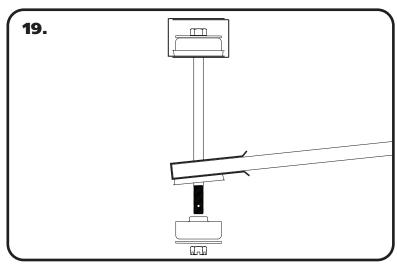
19. You will need to raise the end of the leaf spring up to get the bolt through far enough to get the bottom leaf spring bushing installed. Make sure to jack up the leaf spring by the metal on the end of the spring. DO NOT JACK ON THE COMPOSITE PART OF THE LEAF SPRING.
