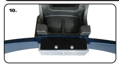
**10.** 78-79 CORVETTE WITH 2 1/2" LEAF SPRING! Position the leaf spring/clamping block in the OEM location with the ends of the leaf spring pointing downward. THE CENTER LOCATING PIN NEEDS TO BE INDEXED INTO THE HOLE OF THE HOUSING.
