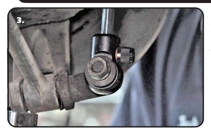
**3.** Jack the trailing arm up to align the shock eyelet with the OEM stud. Attach the shock eyelet to the OEM shock stud. To ease adjustment, position the adjuster knob to the front of the car. Use the OEM hardware to attach it. Torque the nut to 40 ftlbs.
