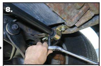
**8.** Again, the mounting holes need to be closest to the bend off the sway bar.. Install a 5/16" Lock Washer & 5/16" Flat Washer on (2) 5/16"x 1" Hex Bolts. Insert the hardware through the OEM swaybar mounting holes, threading the hardware in to the mount. Do NOT tighten the mounting hardware at this time.
