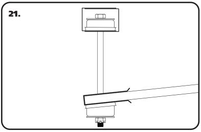
**21.** While holding the bushing and washer in place, thread the 1/2"-20 slotted hex nut on the bolt sticking through the bushing/washer. Thread the nut up the bolt until the cotter pin hole lines up with a slot in the nut.
