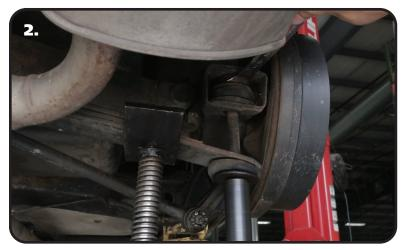
**2.** Use the jack to raise one end of the leaf spring enough to take tension off the leaf spring linkage bolt. Remove the linkage. Slowly release the jack. Repeat on the other side.
