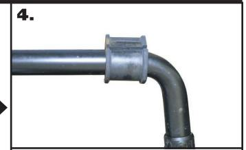
**4.** Open the Sway Bar Bushing at the split and slide it **OVER** the Delrin Liner. Do this on both Delrin Liners.
