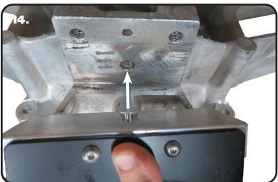
**14. 80-82 CORVETTE!** Position the clamping block in the OEM location with the side plate to the REAR of the car and pointing down. THE CENTER LOCATING PIN NEEDS TO BE INDEXED INTO THE HOLE OF THE HOUSING.
