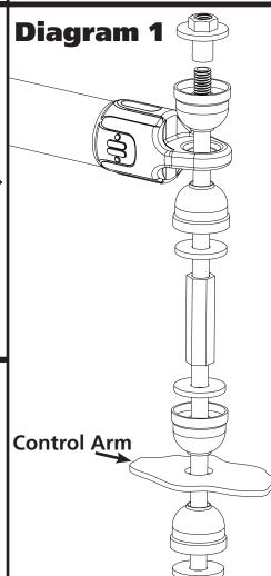
Tighten the end link barrel nut until it is flush with the end of the bolt, and then tighten it 2-3 more complete rounds.
