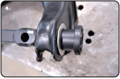
**Note:** The Delrin is self-lubricating, no lubricant is needed.
