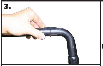
**3.** Open the Delrin Liner at the split and slip it over the Sway Bar. Position it in the area that the bushing will ride based on the location of the stock swaybar. Do this on both ends of the swaybar.
