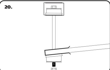
**20.** Slip the lower leaf spring bushing on the threads of the bolt sticking through the leaf springs, followed by the 1/2" ID x 2 OD washer.
