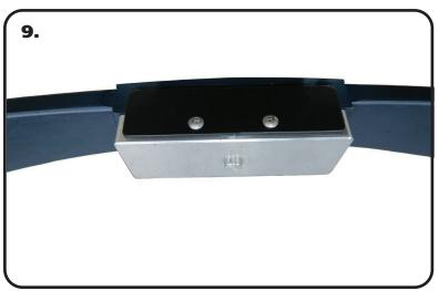
9. 78-79 CORVETTE WITH 2 1/2" LEAF SPRING! Slip the clamping block assembly on the bottom side of the leaf spring, aligning the locating pin with the hole in the clamping block assembly. The clamping block assembly needs to be installed on the leaf spring with the side plates going on each side of the leaf spring. The locating pin in the clamping block should be pointing down away from the leaf spring. The leaf spring is mounted in the car with the ends curving to the ground.
