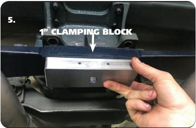
**5. 63-78 CORVETTE WITH 2 1/4" LEAF SPRING!** The kit contains a 1" thick clamping block that needs to be positioned between the composite leaf spring and OEM clamping plate. The clamping block has a center hole that the leaf spring pin will nest into. The pin of the clamping block will be pointing down.
