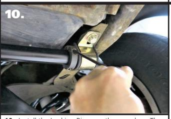
**10.** Install the Locking Rings on the sway bar. They will be positioned against the inside of the sway bar bushings. You will need to disassemble the locking rings to install them on the sway bar. Tighten the hardware with a hex wrench.
