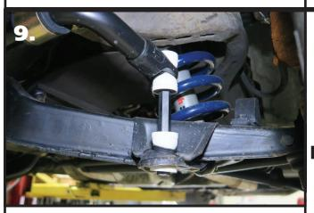
**9.** Install the End Links using **Diagram 1** as a reference. Install both end links before tightening the end link hardware. Tighten the end link barrel nut until it is flush with the end of the bolt, and then tighten it 2-3 more complete rounds.
