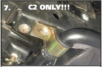
**7. C2 ONLY!!!** The C2 Corvette requires a Spacer to be used between each Sway Bar Bushing and the frame. Be sure to get the offset the same direction as the bushing strap. The holes should be offset toward the bend of the sway bar.
