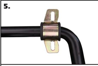
**5.** The Bushing Straps have the mounting holes that are offset. **The Mounting Holes need to be closest to the bend of the sway bar.** Slip the Bushing Straps over the Sway Bar Bushings.
