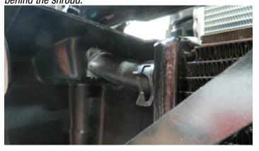
102. Attach the LTR to WP hose to the water pump and secure with a hose clamp from Bag # 3.
