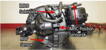
51. Make sure the IMRC harness is completely disconnected from above locations and remove the manifold. Clean the cylinder head flanges as needed and tape up the ports to prevent debris from falling into the ports.
