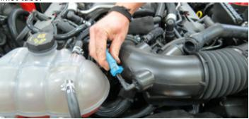
35. Disconnect the brake aspirator hose from the manifold PCV hose.
