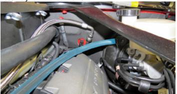
95. Route the Aspirator to Manifold hose under the heater hose and attach to the fitting on the supercharger nose.
