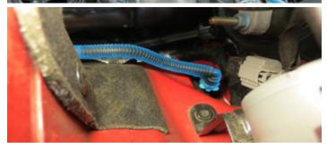
38. Using a hose clamp tool and pliers, remove the brake aspirator hose from the intake manifold.
