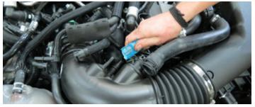
34. Remove the additional brake aspirator hose from the air inlet tube.
