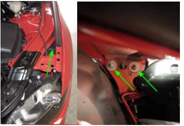
25. From within the wheel well remove the fascia retention assembly that the nuts were removed from in the previous step. Pull downward until the until the plastic pin no longer retains the assembly. Remove from vehicle, ensuring to distinguish between passenger and driver side.
