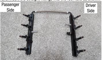
73. Apply 0-ring lube to both ends of the supplied fuel injectors, then install them into the supplied fuel rails. oriented so the electrical connectors will face away from the supercharger.
