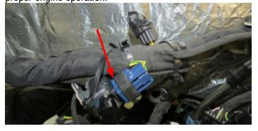
53. Tape up the end of the two (2) IMRC position sensor plugs and secure plugs to the main harness out of the way. These will not be reused.
