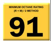
91 octane or higher gasoline is required at all times. If your vehicle has been filled with anything less, it must be run until dry and refilled with 91 or higher octane gasoline twice prior to installation.
