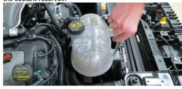
55. Position the coolant reservoir tank out of the way to access the drive belt tensioner.
