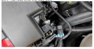
113. Open the fuse box and using a 10mm socket, attach the "Power Supply Wire" on the Water Pump/EVAP Harness to the power terminal on the fuse box.
