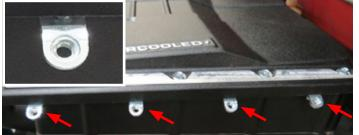
71. For proper bracket alignment, test fit the side covers onto the brackets using eight (8) M6 X 25mm bolts from the side cover kit. While pushing the side covers forward, fully tighten the bracket bolts. Once all brackets are aligned and tightened, remove the side covers.
