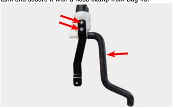
107. Connect the Water pump to Surge tank hose to the water pump and secure with a hose clamp from Bag #3.
