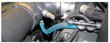
122. Connect the 90° fitting on the supplied driver side PCV hose to the driver side valve cover. Connect the other end to the fitting on the silicone elbow.
