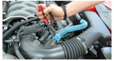
32. Remove the brake aspirator hose from the air inlet tube.
