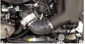
121. Connect the brake aspirator to the lower fitting on the silicone elbow.
