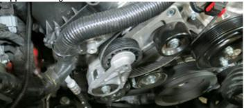
64. Using the M8 x 20mm bolts and M8 washers supplied in Bag # 2, install two idler pulleys to the tensioner bracket. The top idler pulley is 65mm and the lower idler is 76mm. Add a small amount of blue thread lock fluid to the threads ONLY, do not allow excess thread lock fluid to drip onto the pulley's bearings. Torque the bolts to 18 ft-lbs.
