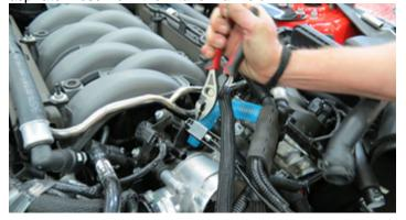
39. Remove the brake aspirator hose assembly from the brake booster and set aside as it will be reused later.
