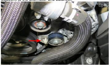
60. Remove both the engine cover bolt using a 10mm socket and the bolt through the ear of the alternator using a 15mm socket.
