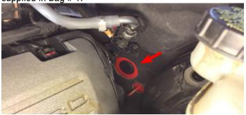
41. Remove the passenger side PCV hose from the valve cover and the intake manifold.
