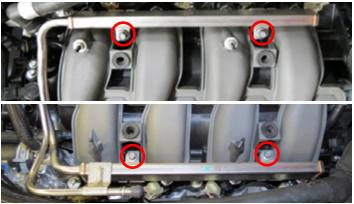
49. Using an 8mm socket, remove six (6) manifold bolts.
