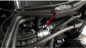
87. Remove the evap solenoid from the factory manifold. Install the solenoid onto the bracket using the factory rubber grommet. Connect the hoses. Put the evap in position and leave the bracket loose until the supercharger installation is complete.
