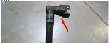
111. Attach the 90° fitting onto the supplied 1/2" Cadbar hose. Connect the quick connect fitting to the passenger side valve cover and the other end of the hose to the barb on the supercharger nose.
