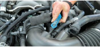
33. Remove the driver side PCV hose from the air inlet tube.
