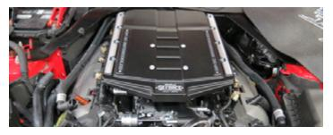
80. Mount the fuel rails and move them away from the supercharger to access the supercharger manifold bolts. Secure the supercharger manifold to the cylinder heads using a 10mm swivel socket to install ten (10) M6 x 30mm intake manifold bolts supplied in hardware Bag # 1. Using the torque sequence below, torque the bolts to 8 ft-lbs.
