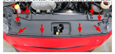
19. Remove six (6) bolts securing the top of the fascia using an 8mm socket.
