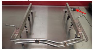
76. Apply fuel resistant thread sealer to the threads of the fuel pressure sensor adapter. Thread the adapter into the supercharger fuel rail until snug. **Ensure not to overtighten and strip threads.** Apply the same thread sealer to the fuel pressure sensor and thread it into the adapter. Prevent the adapter from twisting in further with a second wrench. Optionally continue to twist the sensor once snug until it aligns with fuel rail.
