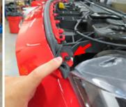
21. Remove sixteen (16) bolts and six (6) push pins securing the splash guard using a 7mm socket and a panel puller. Remove the splash guard and set aside.
