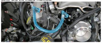
42. Disconnect the throttle body connector.
