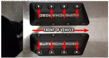
132. Place the evap in position for the coil covers. TIP: Place the bolts through the coil covers first, then feed the bolts into the evap bracket. Then thread the bolts into the supercharger coil cover brackets.
