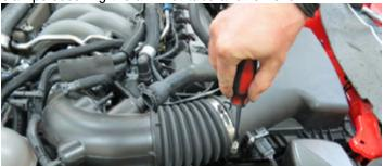
37. Disconnect the EVAP connectors and fully remove the EVAP hose .
