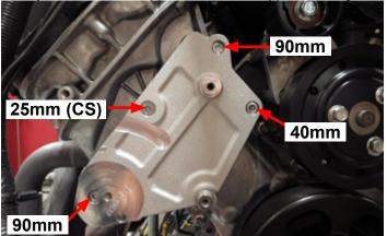
(NOTE: When installing the countersunk bolt, place the .045" thick brass spacer between the bracket and the front engine cover if the hole was drilled and tapped by the factory.) Apply blue thread lock fluid to threads and loosely install the following four (4) bolts from Bag # 2,
