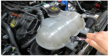
90. Install the supplied coolant bleed hose and secure with the factory hose clamps.
