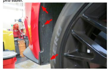
23. There is an additional push pin located just above the tire that needs to be removed.
