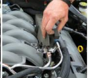
45. Disconnect eight (8) fuel injector connectors.
