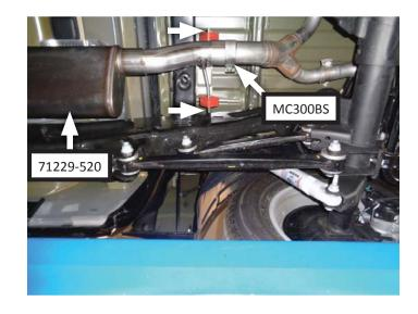
8. Place gasket (removed step 5) between muffler and factory pipe then hang muffler wire hanger into rubber isolator. Connect grounding wire to muffler.
