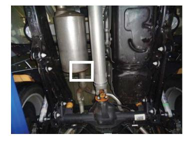
4. Remove bolts attaching muffler and front pipe. Remove grounding wire from muffler.
