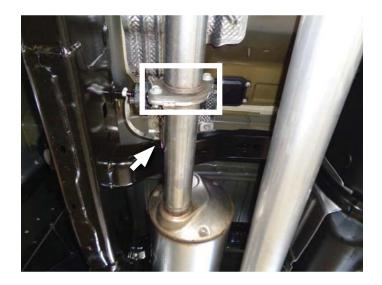
5. Remove muffler wire hangers from mounts, then remove cut out muffler section from factory exhaust system. Remove gasket from factory muffler inlet and retain for re-use.
