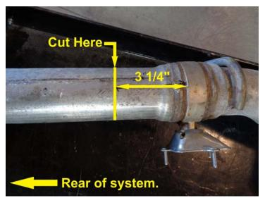
On the passenger side of the system, Measure back 3 ¼" from the cast body of the exhaust valve and make a mark. Using a hacksaw or sawsall, cut the pipe through on this mark. After cutting, remove any burrs from the end of the pipe using a file or die grinder.
