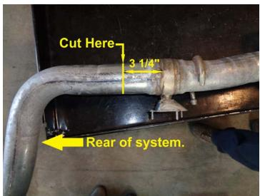
On the driver's side of the system, measure back 3 1/4" from the cast body of the exhaust valve and make a mark. Using a hacksaw or sawsall, cut the pipe through on this mark. After cutting, remove any burrs from the end of the pipe using a file or die grinder.
