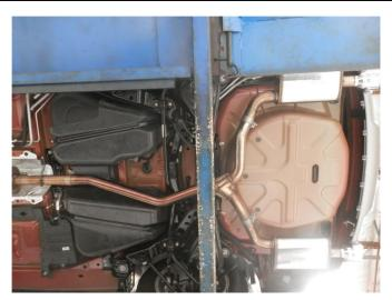
**Step 3.** Next loosely attach the Y-Pipe Assembly and both Muffler Assemblies using the supplied 2.50" clamps. Engage all welded hangers to the rubber insulators.
