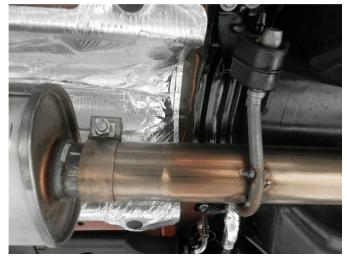
**Step 2.** Begin installation of the new system by fastening the Extension Pipe Assembly inlet to the resonator outlet pipe you just cut using the supplied 2.25" band clamp. Engage the welded hanger to the OEM rubber insulator. Leave all clamps loose for the final adjustment of the complete system.
