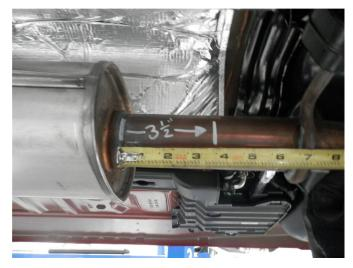
**Step 1.** To remove the OEM exhaust system you will need to cut the pipe 3.50" rearward of the stock resonator as shown. Deburr the freshly cut pipe. Working front to rear disengage all welded hangers from the rubber insulators and remove the system. Do not discard the or damage the rubber insulators as they will be used to mount the new system.
