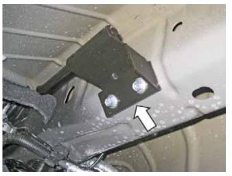
6. Remove the two (2) IRS sub frame mounted exhaust hangers from the stock exhaust system and slide them onto each side of the ROUSH exhaust.
