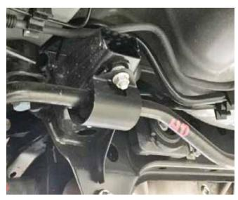
Locate the template onto the rear chassis sub frame as shown in the pictures below and mark the drill holes with a center punch. Use the same template to mark the holes on both the RH and LH sides of the vehicle.
