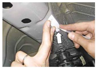
3. Drill all four (4) pilot holes that were marked in the previous step with a 1/8" drill bit followed by a 17/32" drill bit.
