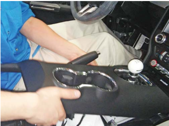
22. With the emergency brake fully engaged, lift the top portion of the center console up and unplug the connectors for the key fob detection circuit and for the cup holder lighting (if equipped). Pull back on the center console to release the clips.
