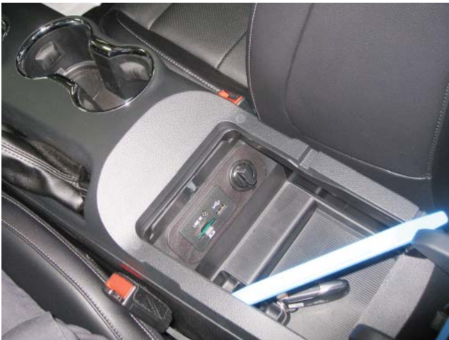
23. Release the clips for the shifter trim bezel and remove the top section of the center console from the vehicle.
