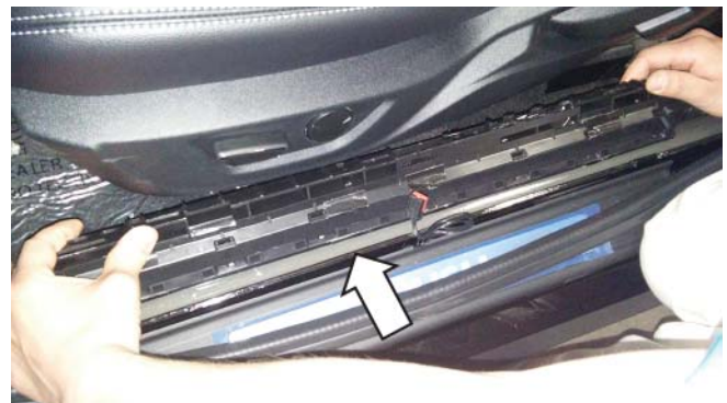
16. Route the active exhaust wire harness along the outside of the factory wiring harness in the wire harness housing. Close the wire harness housing and apply new sections of tape to secure it closed.
