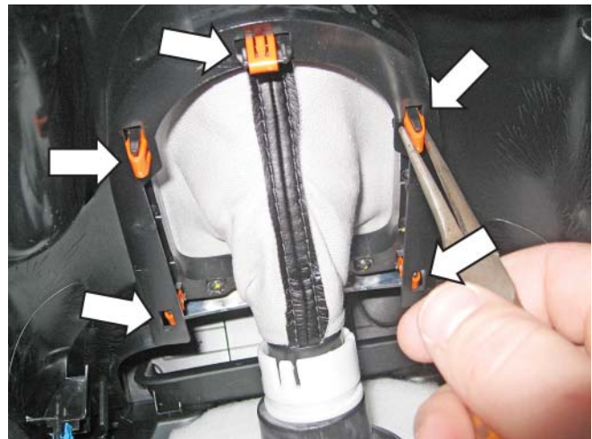
23. Release the clips for the shifter trim bezel and remove the top section of the center console from the vehicle.
