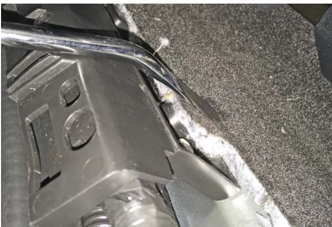
15. Remove the plastic push pins with trim removal tool.
