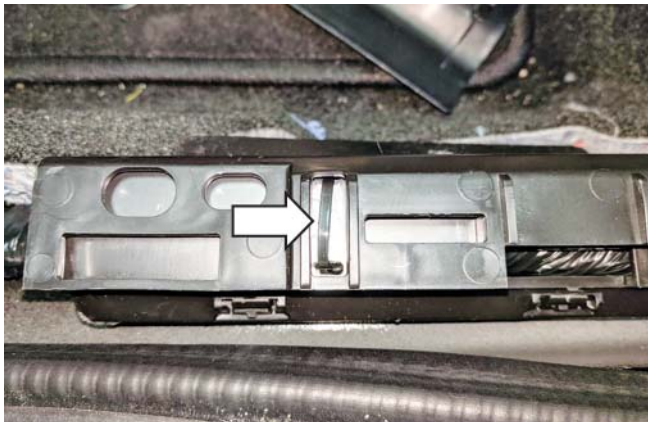
15. Remove the plastic push pins with trim removal tool.
