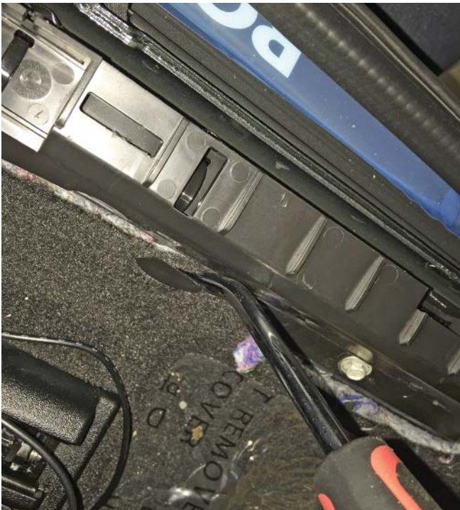
14. Remove the zip ties from the door sill cover.
